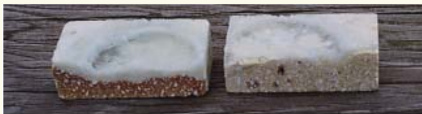
Conventional silica Erosion depth: 6.5–7 mm Penetration depth: 3–5 mm
